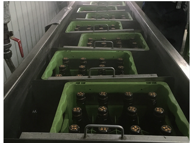
A Sake That Lives: High-Vacuum 'Bottle Pasteurization'
